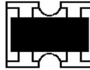
4.2 ±5% Tolerance of 4S02、4S03 size: the first two digits are significant figures of resistance and the third denotes number of zeros following .
